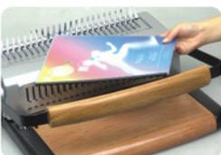
When all the punched sheets are loaded onto the plastic comb, release the *Binding Handle* to its original position to close the plastic comb completely. You can now remove the bound booklet and enjoy your finished work.
