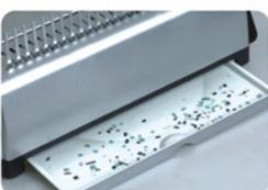
Take out the *Waste Tray* from the back side of the machine. For best results, empty the tray regularly.
