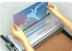
Take out the punched sheets from the *Punching Channel* and position them vertically in the open comb. Locate the punched holes over the open comb fingers and rotate the sheets forward onto the comb.
