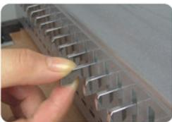
These punch dies can be disengaged as required to suit the size of paper being punched. To disengage a punch, simply pull out the desired *Punch Selector* by hand. To re-engage, simply press it to the original position.
